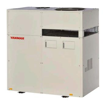
Using natural gas, the CP35D1's highefficiency generator provides 35 kW of electrical power. The engine heat is captured and heats water at a rated temperature of 176°F for immediate use or storage in your facility. Excess electricity production may be sold back onto the grid in certain states, creating a credit on your electric bill.
